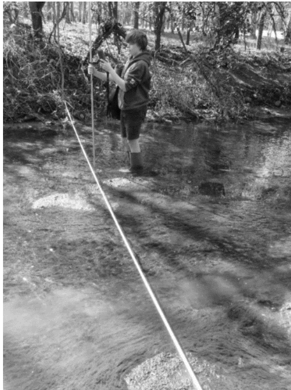
Fig 1. Setting up flowmeter and tag line with measuring tape (Eustace Barnes)
